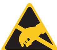
This symbol appears on the main board of the unit and indicates that the board contains static sensitive components. Suitable anti-static precautions must be taken when handling the board.
