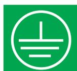
This symbol indicates the Safety Earth stud (see section 6.2.1). This is for grounding cable screens and should not be connected to 0V or signal earth.
